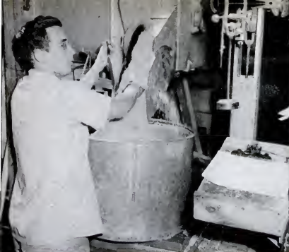
Sawdust-like mix of ground wood and resin powder pours into container as worker watches a scale balance. Mixer overhead continuously adds resin to wood in controlled proportions.
